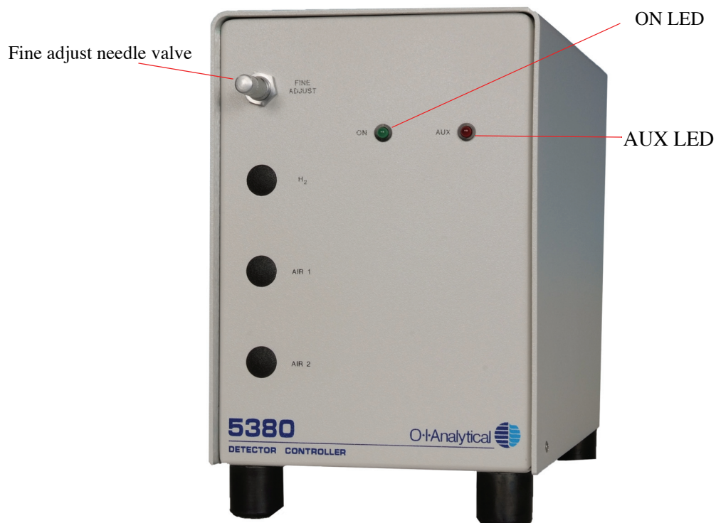
Figure 2.4. Model 5380 Detector Controller, EPC Ready for GCs with Electronic Gas Flow Control
